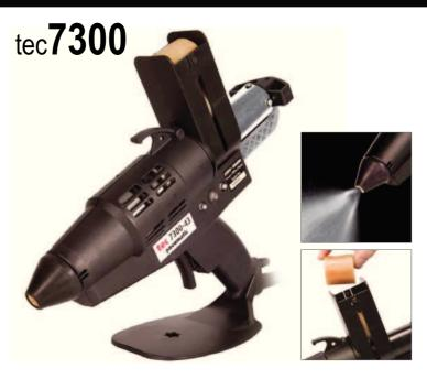
Extremely robust, 43mm (1¾") spray glue gun. Non-toxic adhesive spray system, sprays hotmelt at any angle, adjustable spray pattern to cover large areas. Apply hotmelt to heat sensitive substrates without damage. Speed loader to reduce downtime, plus power-on light. 8 bar (120psi) 85 l/min (3 cfm) air supply required.
